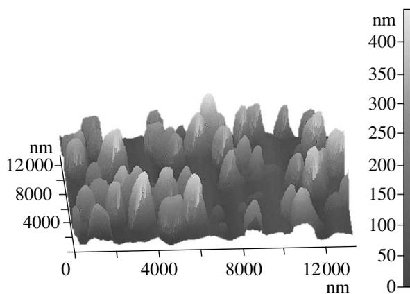
**Fig. 3.** Isometric image of the  $\text{SiO}_2$  surface with etched ion tracks filled with Cu.
