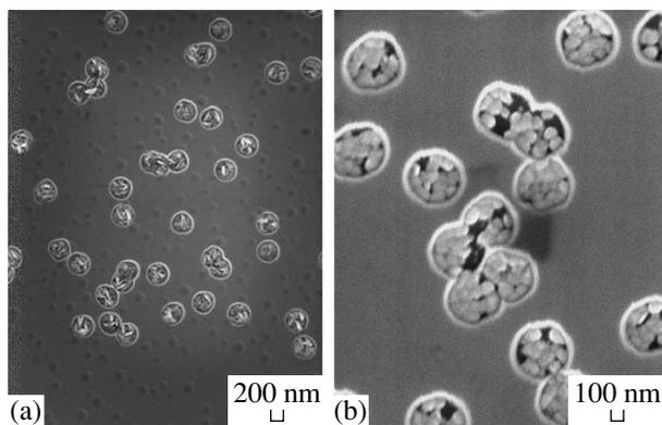
**Fig. 2.** SEM images of  $\text{SiO}_2/\text{Si}$  structures with (a) Cu and (b) Ni nanoclusters in etched ion tracks in a silicon dioxide layer.
