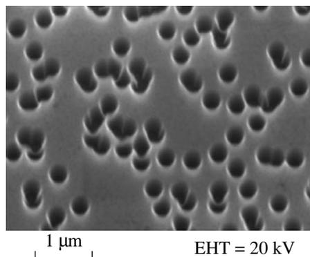
Fig. 1. SEM images of ion tracks, which are conical nanopores after etching.
