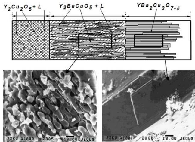
**Fig. 7** Diffusion layers of  $\text{Y}_2\text{BaCuO}_5 + \text{L}(\text{BaCuO}_2)$ .
