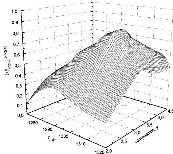
**Fig. 2** Plot of  $\langle S_{\text{mgain}} \rangle / \langle S \rangle$  vs  $T$ ,  $y$  -  $(\text{Y}_2\text{Cu}_2\text{O}_5 + y\text{BaCuO}_2)$  for  $\text{YBa}_2\text{Cu}_3\text{O}_{7-\delta}$ .
