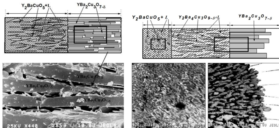
**Fig. 5** Diffusion layers of  $\text{Y}_2\text{BaCuO}_5 + \text{L}$  ( $\text{BaCu}_{1.8}\text{O}_z$ ) system.
