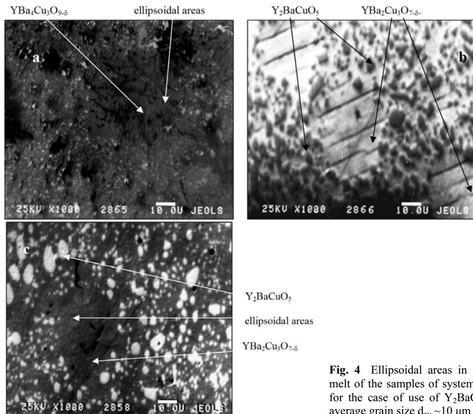
**Fig. 4** Ellipsoidal areas in the tempered solution – melt of the samples of system II (a), I (b), and III (c), for the case of use of  $\text{Y}_2\text{BaCuO}_5$  and  $\text{Y}_2\text{Cu}_2\text{O}_5$  with average grain size  $d_{av} \sim 10 \mu\text{m}$  in the initial furnace.
