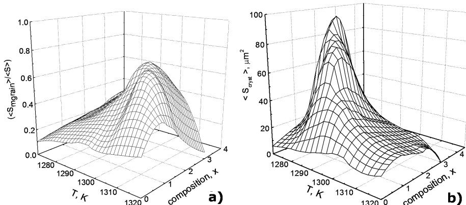
**Fig. 1** a) Plot of  $\langle S_{\text{mgain}} \rangle / \langle S \rangle$  vs  $T$ ,  $x$  -  $(\text{Y}_2\text{BaCuO}_5 + 3\text{BaCuO}_2 + x\text{CuO})$  for  $\text{YBa}_2\text{Cu}_3\text{O}_{7-\delta}$ . b) Plot of  $\langle S_{\text{cryst}} \rangle$  vs  $T$ ,  $x$  -  $(\text{Y}_2\text{BaCuO}_5 + 3\text{BaCuO}_2 + x\text{CuO})$  for  $\text{YBa}_2\text{Cu}_3\text{O}_{7-\delta}$ .
