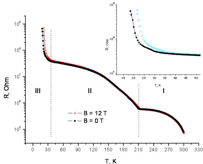
**Fig. 1:** temperature dependences of resistance in zero magnetic field and magnetic field of 12 T.
